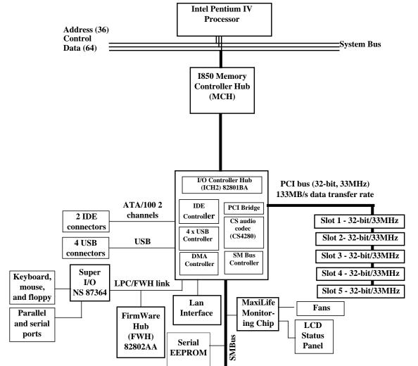
Figure 2-8System Block Diagram Using ICH2
